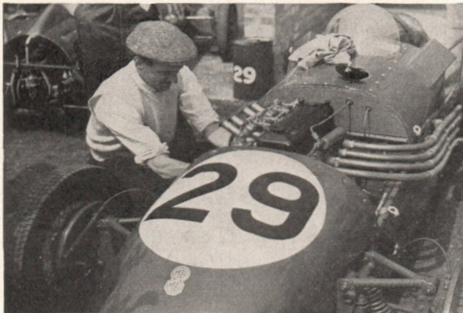
"500" FOUR: Spotted at a recent Silverstone club meeting—H. H. G. Monk's M.B.M.G., with P-type M.G. engine reduced by short-throw crankshaft to 496 c.c. and using four Amal carburettors inclined at 45 degrees.
