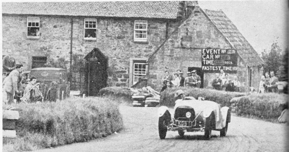
**ROVER SPECIAL:** (Left and Right) 115 m.p.h. on overdrive is achieved by Jimmy Gibbon's Special, which has a basically P3 Rover frame and front suspension, Javelin-cum-Rover rear end, and a choice of two much breathed-upon Land Rover engines. Picture opposite shows the car at Turnberry; that on the right at Prescott.
