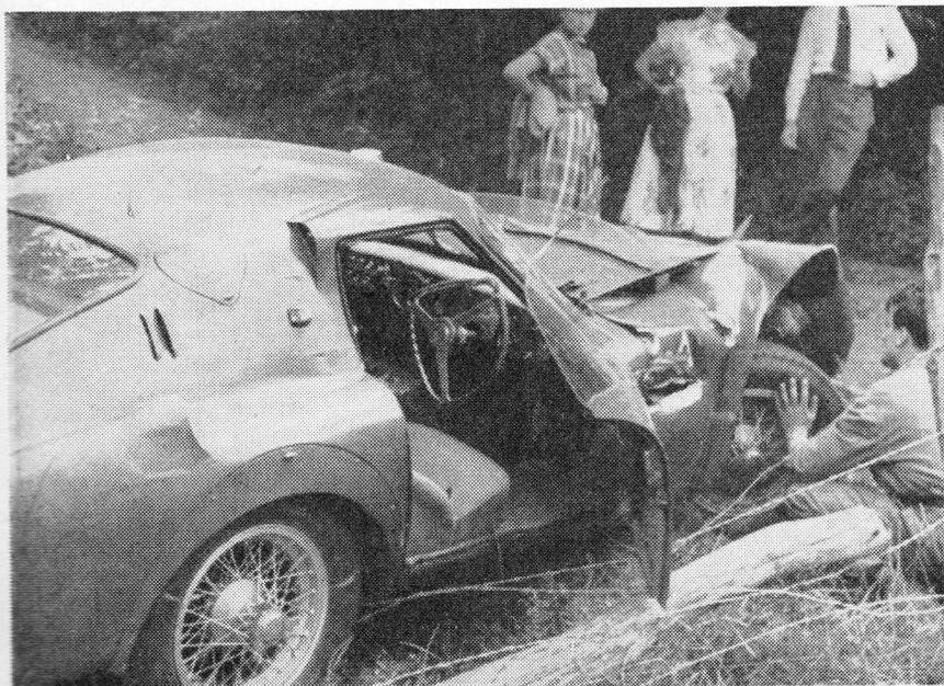
*KLING CRASH: This happened at Nürburgring during tests for the forthcoming 1,000 kilometres race, when the 3-litre Alfa Romeo driven by Karl Kling crashed into a wall after believed steering rod breakage. The driver was only slightly injured.*
