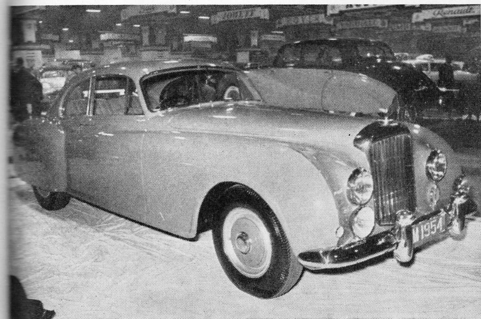
LUXURY SALOON: (Above) Latest version of the very fast Bentley "Continental", which, with 4½-litre o.h.v., six cylinder engine, achieves a comfortable 115 m.p.h.
