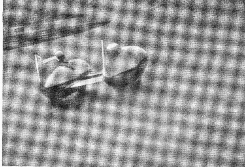
BISILURO: Piero Taruffi's twin-fuselage Tarf 500 at Montlhéry, setting up new Class I records which it lost a few days later to the Arnott illustrated below. (Left) A glimpse of the 4-cylinder Gilera engine, installed in the right-hand boom.
