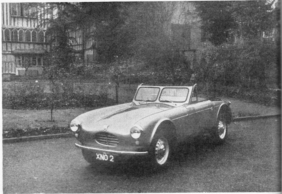
(Above) Three-quarters front view of the car. The wind-up windows have fixed frames. (Below) The steel tubular superstructure to which are secured the Fibreglass shell and panels, is seen in this picture taken during assembly.
