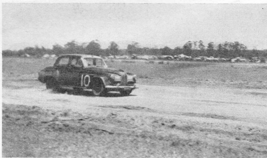
ROUGH GOING: Tommy Sulman's stock Humber Snipe saloon kicks up the dust on a fast section of the Mt. Druitt circuit. The car travelled the entire 24 hours without any needs other than fuel, oil, water and tyres, finishing in third place.
