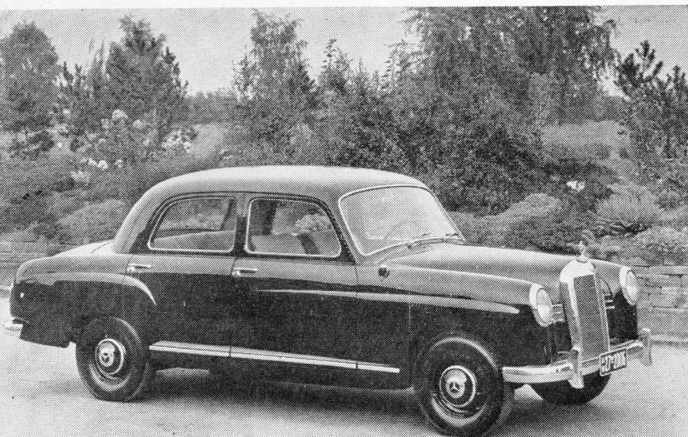
DIESEL: (Left) The Mercedes-Benz, Type 180D with 1.7-litre four-cylinder compression ignition engine achieves 45 m.p.g. and 68 m.p.h. in effective manner. (Above) A 180D with bonnet raised, revealing the readily accessible power unit.
