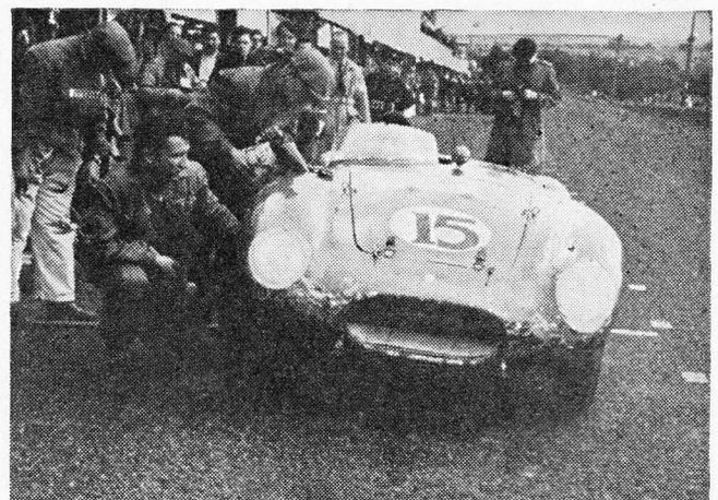
Nearside wheels renewed, the offside now receive attention, while oil is poured in via the most accessible filler cap set in the wing.
