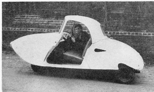
THREE-WHEELED "CLIPPER": The plastic-bodied Allard model has a 350 c.c. Villiers two-stroke engine driving through belts.
