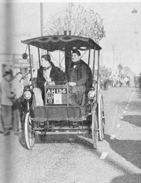
on the long Purley Hill, 18 miles out from Hyde the machine has a coke-fired vertical boiler, and wheels by flat belt.
