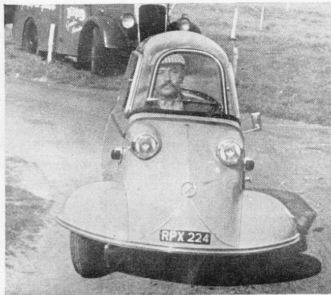
"The engine is easily the best two-stroke I have ever come across". (Above) The 174 c.c. Sachs motor is installed in conventional motor-cycle style. (Left) "No normal driver need ever fear that he will tip up his cabin scooter". Only by excessively fast cornering did Bolster manage to lift an inside front wheel.
