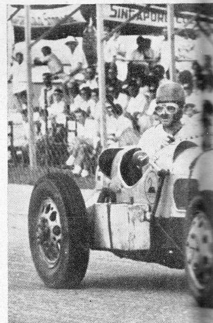
Sidney Anderson of Western Australia (above) in the Johore Grand Prix. Curiously, it is in fact powered by two V-8 commercial units, one in front of the driver, one behind, the driver.
