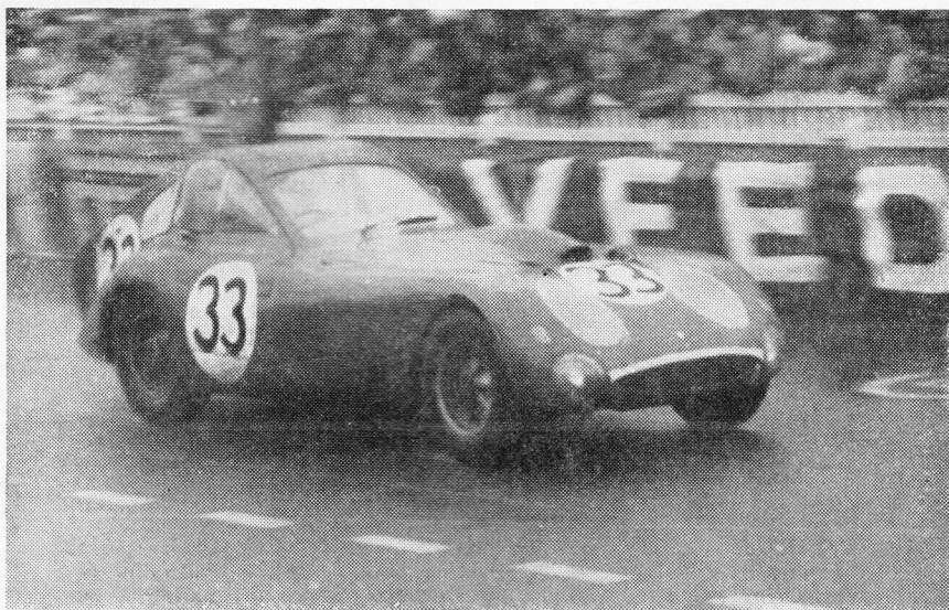
CORRECT DESIGN in the Bristol 450 allows the use of a very small air intake, by virtue of its being located low down at a point of high air pressure.
