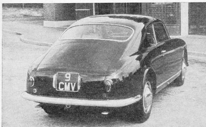
SHAPELY TAIL (Above), although it houses a 17-gallon fuel tank, opens up to reveal (right) a most capacious luggage boot.
