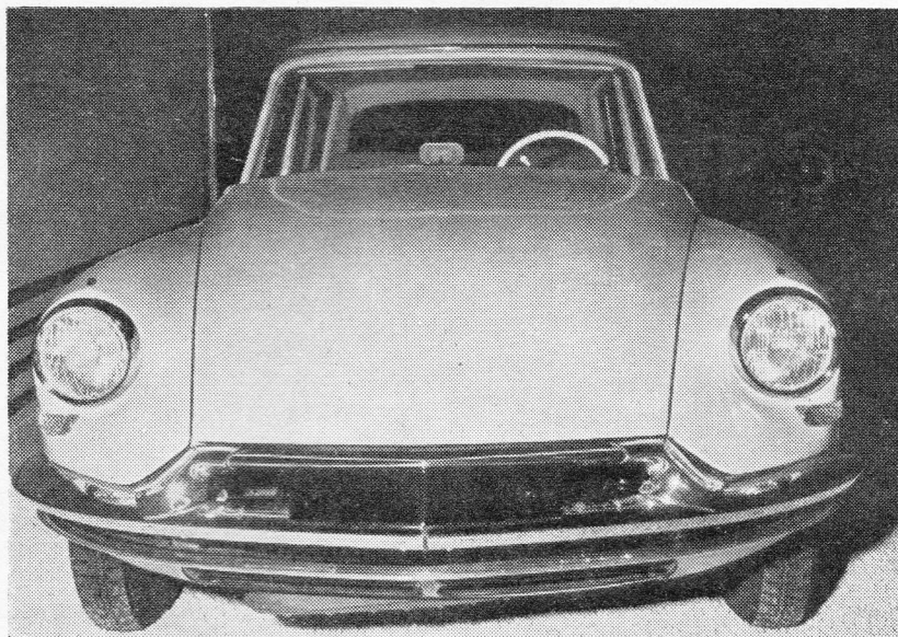
SENSATION OF PARIS: And to be seen at Earls Court on Stand 155, is the highly unconventional Citroën DS19, with 2-litre, front-drive engine, hydro-pneumatic suspension, automatic clutch, front disc brakes and other novelties.
