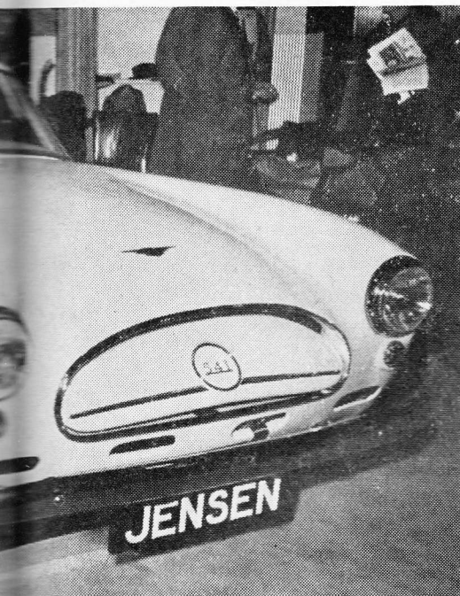
FIBREGLASS is the material for the handsome bodywork of the Jensen 541. The radiator shutter is adjustable.
