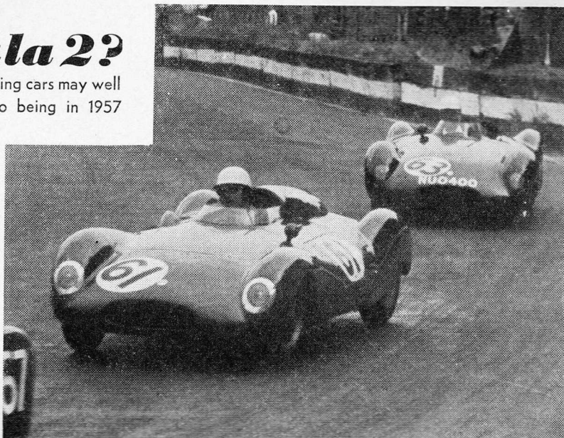
COOPER —Powered by the 1,100 c.c. Coventry Climax unit, this tiny vehicle has frequently triumphed over 1½-litre machines. With the new 1,500 c.c. Climax, due to appear for the coming season, its potency will be even greater.
