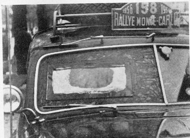
REMEDY for a broken windscreen on the White/McAdam Jaguar was a sheet of glass stuck over the hole with Bostik.
