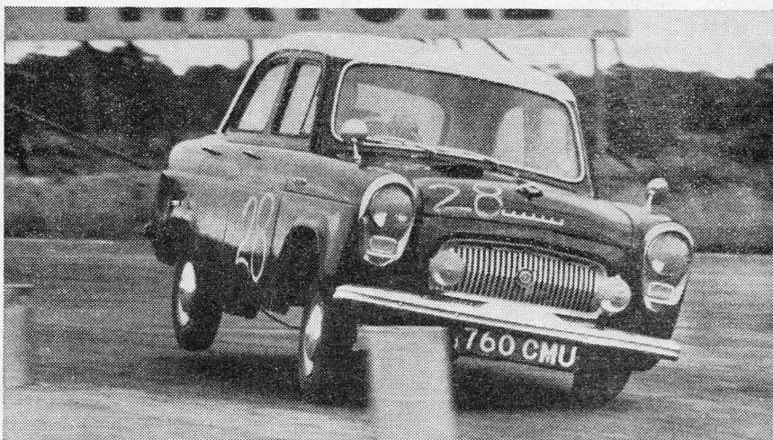
KNEES BEND: Ian Walker's Prefect has an o.h.v. converted engine that produces phenomenal b.h.p. Moreover, he knows how to use it and generally negotiated corners in this manner.
