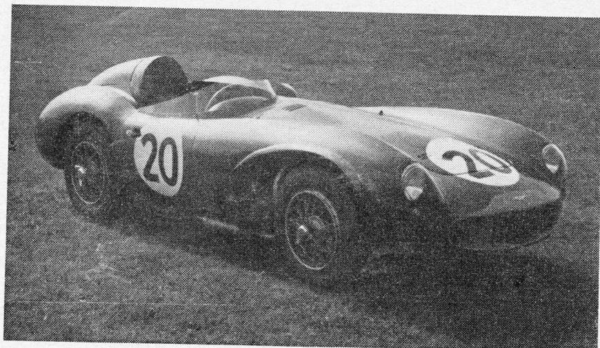
NEW ASTON. Destined for "Le Mans", the new Aston Martin DB3S has re-styled bodywork, the principal features of which are the head-faring and narrower frontal intake. This is the car driven at Rouen by Roy Salvadori.
