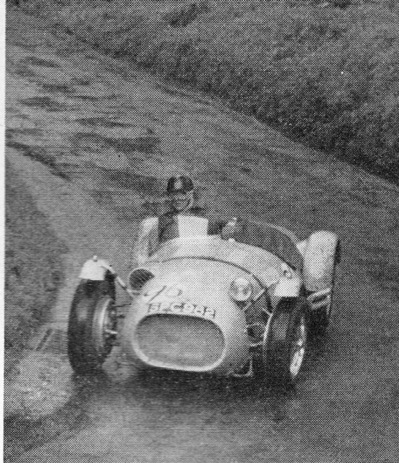
SEEN AT SHELSLEY on 25th August was E. P. Scragg's new Alta-Jaguar, with ex-Formula 2 Alta chassis and D-type engine. The car was built by H.W. Motors.
