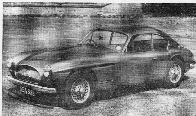
BRITISH BULLDOG: Considerable performance is on tap in the all-fibreglass bodied Jensen 541 (above), which is powered by a 4-litre six-cylinder Austin engine. Its streamlined shape and high gearing give high-speed, effortless cruising.
