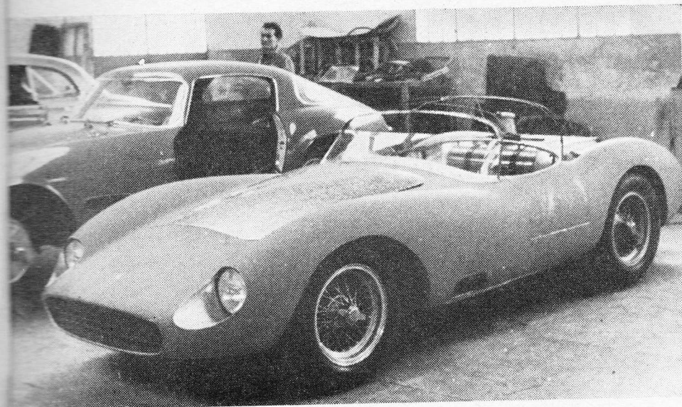
BODIED BY SCAGLIETTI: The latest 3½-litre V12, twin o.h.c. sports Ferrari, seen incomplete, and in its undercoating, at Modena. With 360 b.h.p. under the bonnet, a speed of over 185 m.p.h. is expected.
