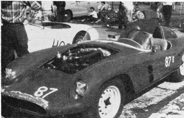
BEARING little resemblance to its original form, but nevertheless an indisputable Triumph TR2, Jerry Barber's shapely machine is fitted with a Devin fibreglass body.
