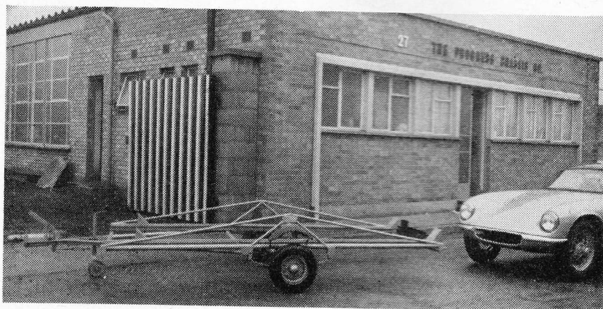
LIGHTWEIGHT trailer for racing cars is produced by the Progress Chassis Co., of Edmonton, London, and costs £72 or £79 10s. with lights and all accessories. It weighs 328 lb. and can carry a car weighing up to 12 cwt. The jockey wheel can be extended to bring the trailer into a drive-on loading position; the car shown is, of course, a Lotus Elite.
