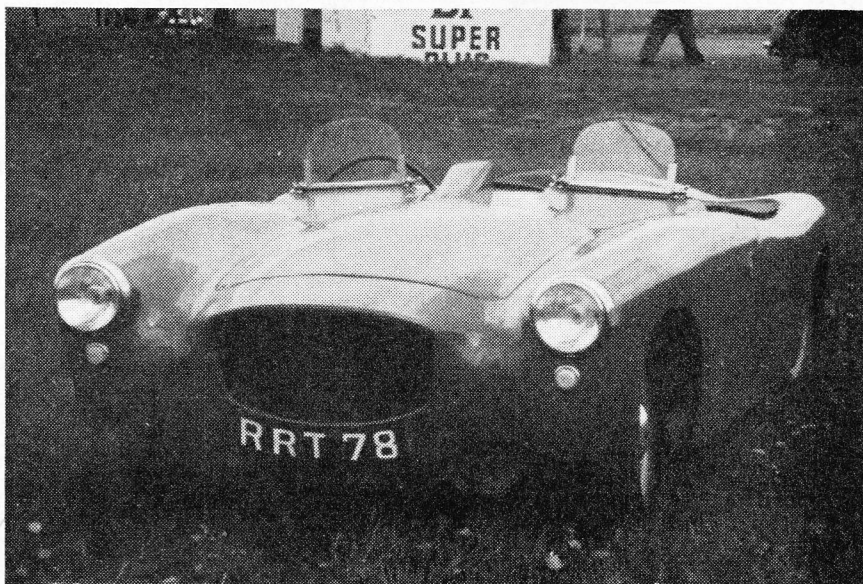
LIKE IT? Perhaps the only wooden car in the country—yes, we mean it—this is powered by a modified Standard Ten unit and has a body of laminated plywood—built, presumably, on small-boat principles. Our photographer saw it at Snetterton during the Allard O.C. sprint recently.
