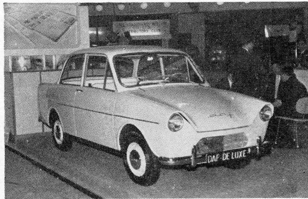
THE OPPERMAN STIRLING (left) sporting runabout is a very pretty little fibreglass-bodied vehicle. All-independent suspension is employed. UNIQUE: The DAF is the first Dutch car since the Spyker. It employs a unique form of belt transmission.
