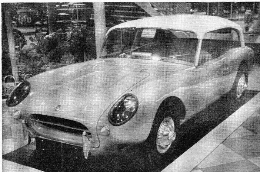
NEW BERKELEY (left)—now a full four-seater. With the three-cylinder Excelsior 492 c.c. two-stroke engine to power it, this should be a popular buy. The engine develops 32 b.h.p. against an all-up weight of 7 cwt. Quite impressive!
