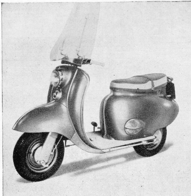
CO-OPERATIVE effort between B.S.A. and Triumph is this new scooter which is available with either a single-cylinder 175 c.c. two-stroke engine, or a 250 c.c. o.h.v. twin. The latter is illustrated installed in the frame.
