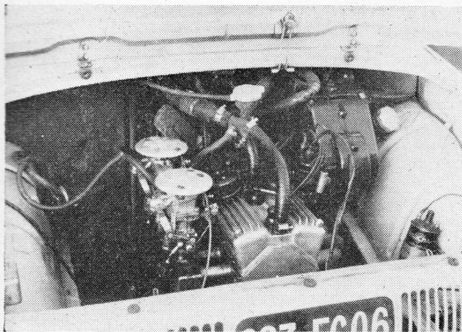
MIGHTY ATOM: A new hemispherical cylinder head (above), produced by M. Colluci in the South of France, is claimed to give the Renault Dauphine 56 b.h.p. at 6,500 r.p.m. The installation is seen (left), with neat, finned valve-rocker cover, and twin carburettors. Cost is approximately £143.
