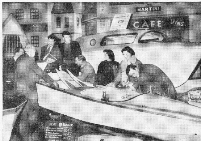
RUNABOUT and cruiser: in the foreground the 14 ft. 6 ins. "Ceabird" resin-glass runabout, and behind the brand new "Cea-Cruiser", a 17 ft. outboard two-berth cruiser.
