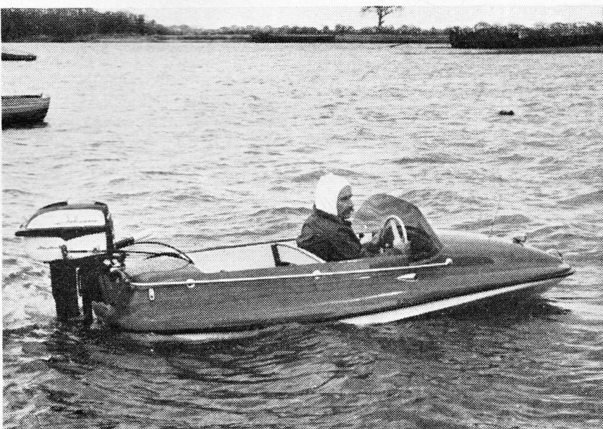
THIS 18 H.P. JOHNSON MOTOR (above), which John Bolster used on his tests, provides enough power for water ski-ing but is still small enough to be started with little effort, with practice, even by a schoolboy.
