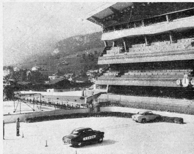
TESTS ON ICE prove the superiority of the new tyres, equipped with studs. Two identical cars were used, the black one wearing B.S.3s. The pictures show a cornering test (left) and a braking test (right).
