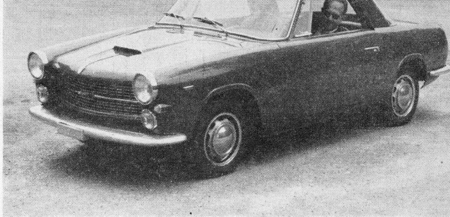
*TINY but purposeful-looking the "Ferrarina" coachwork is by Pininfarina. Disc brakes and overdrive on third and top gears are features of this latest remarkable product of Maranello. The 850 c.c. engine produces 75 b.h.p. at 6,800 r.p.m.*
