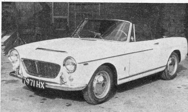
FIAT: For the sportsman there is the Fiat 1500, which uses a 1,491 c.c. overhead camshaft engine to provide a maximum speed in excess of 100 m.p.h. with sporting road-holding and acceleration.
