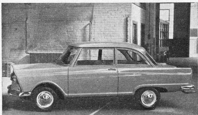
DKW: The DKW Junior, another of the interesting front-wheel drive, three-cylinder, two-stroke engined cars, is now available for the first time in right-hand form. Stand No. 143 houses examples of these entertaining German machines, which have strong "enthusiast appeal".
