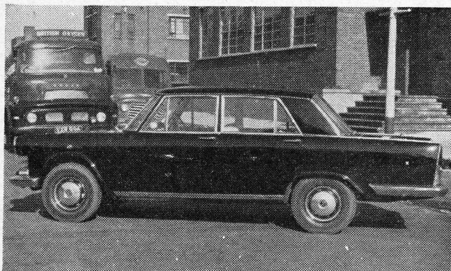
FIAT: Largest of the range is the 2100 saloon, with a six-cylinder engine of just over 2 litres which provides a maximum speed of nearly 90 m.p.h. with a not excessive fuel consumption.
