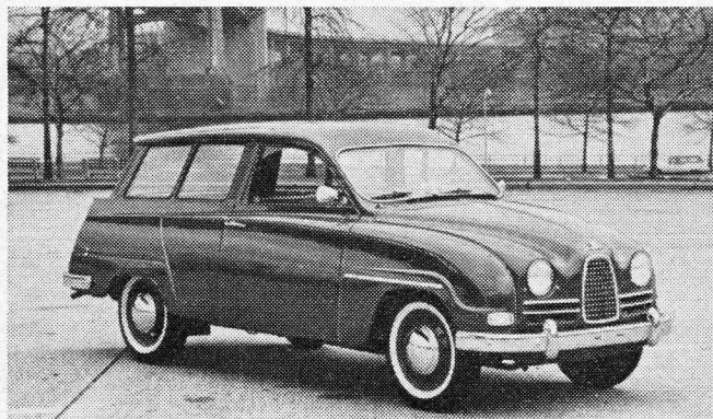
SAAB: Up to seven people and their luggage can be accommodated in the "95" station wagon. Power unit of the Swedish car is a lively 841 c.c., three-cylinder two-stroke engine. Stand No. 152.
