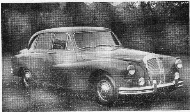
DAIMLER: The well-established 3.8-litre Majestic is unchanged from its previous appearances. Disc brakes are fitted to the car, and it is capable of very high performance. Stand No. 128.
