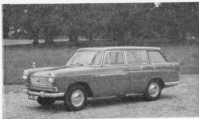
AUSTIN: The A55 Cambridge, the Mark 2 version of which appears again with but detail improvements, employs the B.M.C. "B"-type 1½-litre power unit, and provides comfortable transport for up to five people. Stand No. 102.
