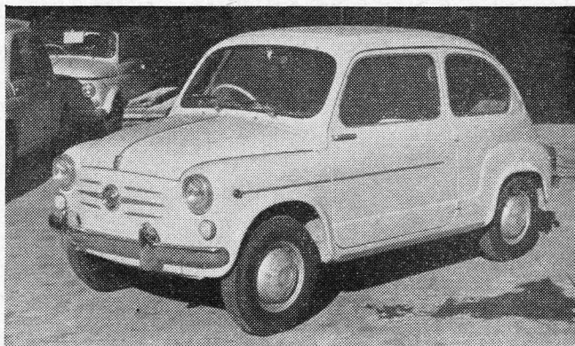
FIAT: Another newcomer this year is the 600D, a development of the tremendously popular 600, which will still be available. Power unit has grown in size to 767 c.c., and there are other changes.
