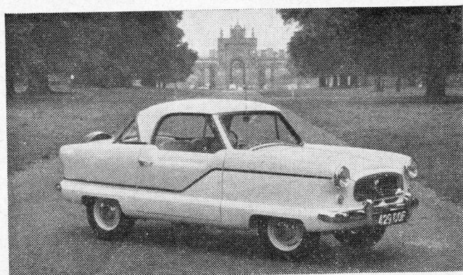
METROPOLITAN: For the customer who likes the American look allied to European compactness. Power unit is the B.M.C. 1½-litre "B"-type engine allied to a three-speed gearbox. A radio is a standard fitting.
