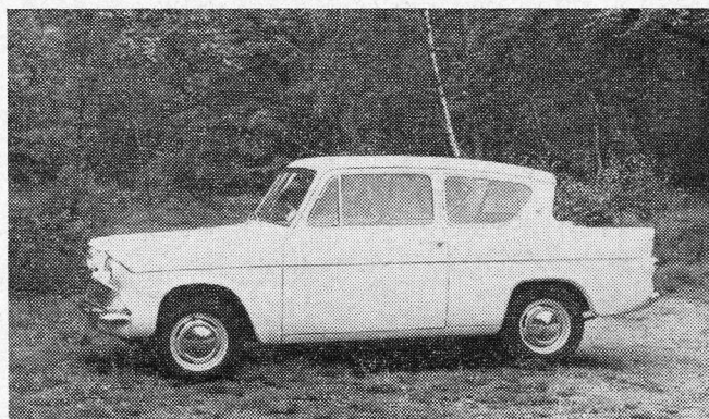
FORD: At the other end of the scale there is the 105E-engined o.h.v. Anglia, with four-speed gearbox (above), while for really cheap motoring there is the Popular (below), last stronghold of the 100E power unit.
