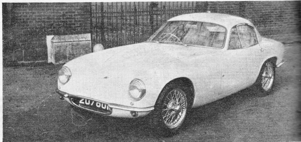
or "DAD 10". Thus, the Coventry Climax engine was in Stage I tune, though with twin carburettors, and a very effective double exhaust system rendered the machine entirely suitable for London. The M.G.A gearbox also had the standard ratios, which would be rather wide for tackling the circuits. Nevertheless, the basic car was identical with the
