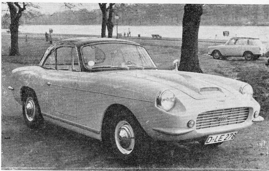
ABOVE: This handsome newcomer is the DKW-Caribbean, an experimental prototype based on a DKW Junior chassis and engine unit with a Falcon Caribbean body shell.
