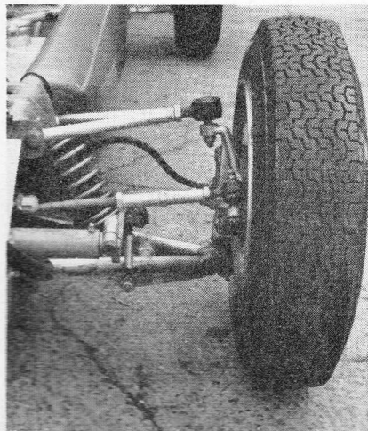
Front suspension: new helical springs, upside-down dampers, longer wishbones.
