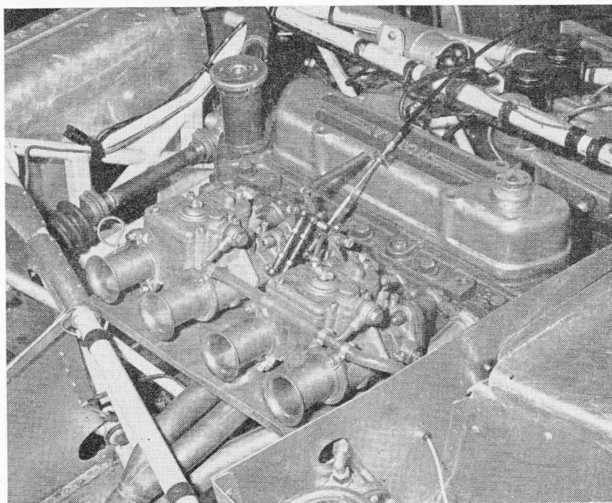
Twin Weber carburettors as fitted to the successful Formula Junior Holbay-Ford engine.
