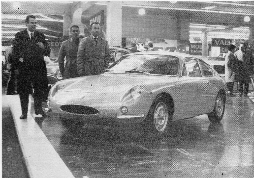
THE SIMCA-ABARTH, a competition-type rear-engined car with 1,300 c.c. engine. This is not the five-bearing Simca unit but an Abarth motor with forged three-bearing crank.
