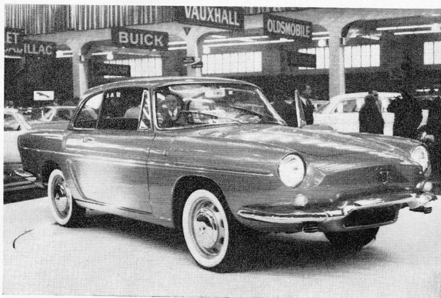
THE LATEST Renault Floride, with sealed cooling system, a five-bearing engine and disc brakes.
