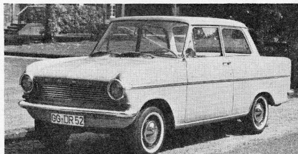
OPEL KADETT. A conventional car recently introduced by the German branch of General Motors, having a 993 c.c. engine developing 40 b.h.p. at 5,000 r.p.m. An all-synchromesh four-speed gearbox is used in this car which has been designed to compete against the Volkswagen 1200.
