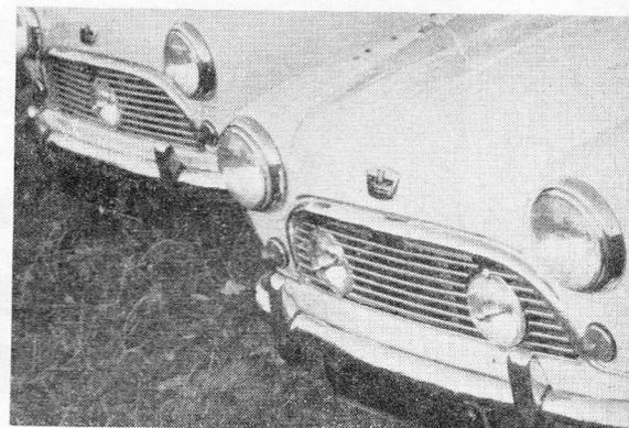
BENELITE GRILLES, 6-51 Lillington Road, Leamington Spa, Warwickshire, now produce a new radiator grille designed for the B.M.C. Mini range. The aim of the design is to provide a neat method of mounting auxiliary lamps in a position where they should not come to any harm!
