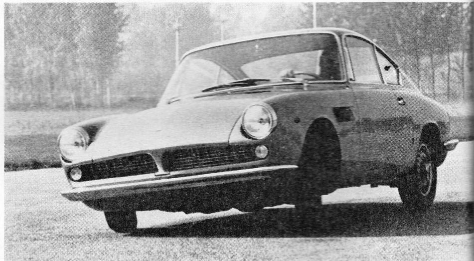
rods. The ventilated disc wheels are of the Rudge-Whitworth knock-off type, and carry 145 x 13 tyres. The body-shell is all-steel, the weight of the complete vehicle being quoted as 780 kilogrammes. Presumably the competition versions intended for Le Mans and other races will have light alloy bodywork. The frame is conventional steel-tube, very much Ferrari in conception, and notably robust.
