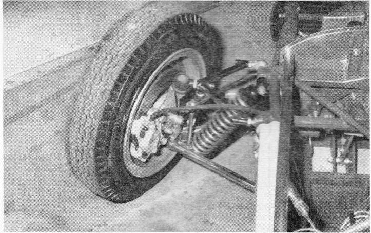
**FRONT SUSPENSION** incorporates adjustable top wishbones
