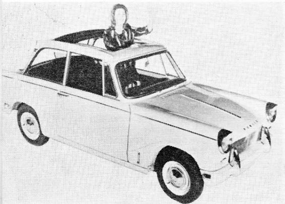
*THE ONLY volume production British car to be fitted with a skylight roof as standard equipment, the Triumph Herald 12/50 was unveiled this week. The 1,147 c.c. engine develops 41 b.h.p. at 4,500 r.p.m. and the car has a claimed maximum speed of over 80 m.p.h.*
