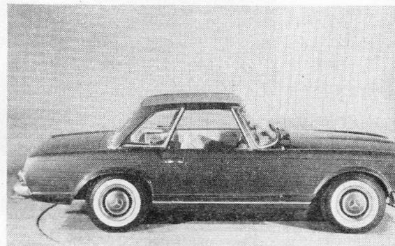
LONG-AWAITED new Mercedes-Benz sports car was introduced this week. Called the 230SL, it is powered by a slightly modified version of the twin-cam, fuel injection, six-cylinder 220SE engine and has a claimed maximum speed of 124 m.p.h. It is available as a Roadster with flush folding soft-top, as a Hardtop Coupé, or a combination of both. It is a very comfortable sports car.
