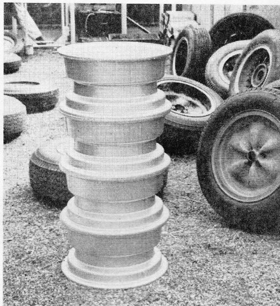
NEVER BE WITHOUT A CAPSTAN. A pile of 7½ in. rim, magnesium alloy Dunlop wheels as used at Aintree by B.R.M. and also destined for the Lotus-Ford "Indy" car.
