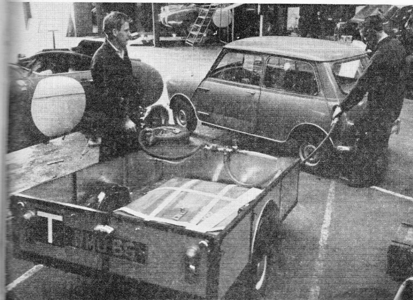
MOBILE BOWSER for use by B.M.C. team (below, left). The collapsible Dunlop tank lies in the bottom of the trailer and can be covered with tyres and other spares when not in use. NOBBY HALL with a cylindrical two-gallon auxiliary fuel tank which will be fitted in the boot of the Mayman/Domleo M.G. 1100 (below, right). This is for use on one section on which a recce has shown that the M.G. 1100 will run a little short of fuel.
