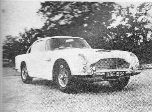
THE NEW Aston Martin DB5 is a 4-litre, 6-cylinder car developing 282 b.h.p. It has a diaphragm-spring twin-plate clutch and though a 4-speed, all-synchromesh gearbox is standard, a 5-speed box is optional.
