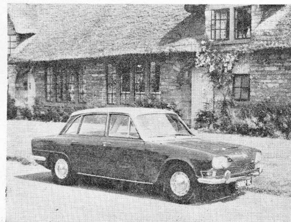
This new car is no sluggard, and can accelerate from rest to 60 m.p.h. in about 14.5 secs. Maximum speed is certainly over 90 m.p.h., probably nearer 95 m.p.h. Roadholding is first-rate, and there is a commendable freedom from roll, which is a compliment to the all-independent springing. The engine is delightfully smooth throughout its speed range, and full marks are given to the splendid all-synchromesh gearbox, with its handy centre-change.
