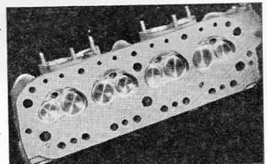
4 separate inlet ports, giving cross flow, developing 20% more power on same c/r than standard with 10% economy and greater smoothness. Mk. II kit with valves and springs, assembled, £68.10.0. Mk. III for 1800 models, £75, with O/S valves & ports.
