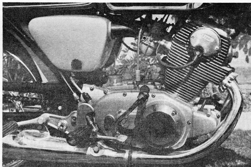
HILLMAN IMP (left). Complete with four persons and stacks of baggage, the little Imp did over 45 m.p.g. on a long Continental trip. EXQUISITE (right). The power unit of the 250 c.c. Honda is a double-o.h.c. twin. It is in unit with the gearbox and boasts an electric starter.
