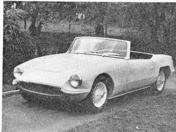
ONLY 100 m.p.h. open two-seater in Europe with fully independent suspension selling in the U.K. for under £1,000 tax paid is the T-type Elva Courier Mk. 4. There are a choice of power units from 1,500 c.c. to 1,800 c.c.
