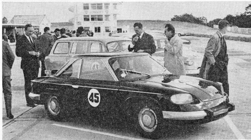
*PANHARD 24 has a distinctive appearance (left). The twin-cylinder car is capable of a sustained 90 m.p.h.*
