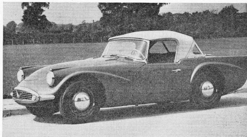
THE DAIMLER SP250 has a 2½-litre V8 **DAIMLER SP250** engine which is smooth and silent as well as developing a great deal of power right up the revolution range. The chassis is entirely conventional, passing beneath the rear axle, which is located by flat semi-elliptic springs, and the port end is on wishbones and helical springs. The body is of glassfibre construction, with winding windows in the doors. The car is capable of a timed speed well in excess of 120 m.p.h.
