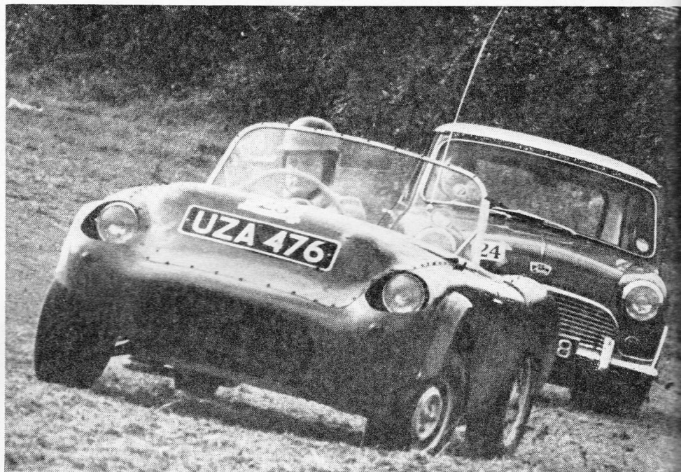
DICKIE LOVELL-BUTT in his Berkeley ahead of Dermot Carnegie's Austin Mini in the I.M.R.C. Autocross on 14th September. The Berkeley is fitted with a Mini engine, 10-in. wheels and Mini front suspension. Very interesting!
