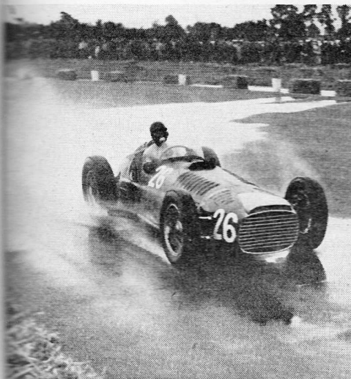
V16 B.R.M., a supercharged 1½-litre Grand Prix car of the early post-war formula. Although the existing 1½-litre engines could be supercharged, unsupercharged 3-litre power units are more likely.
