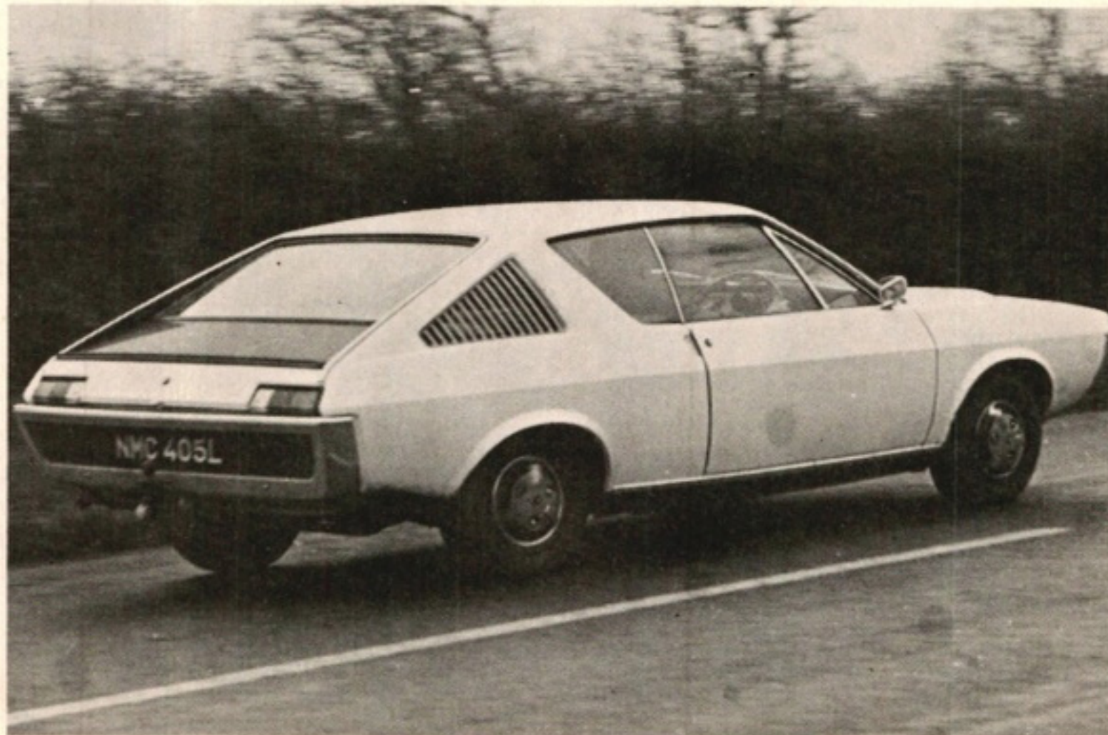
The luggage boot gives useful space and the sloping rear panel lifts for access.
